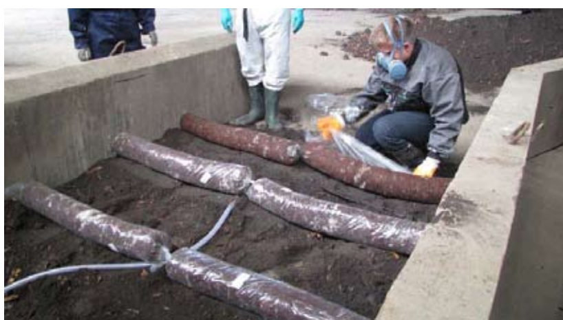
Figure 2. Application of pregrown fungal tubes on TNT contaminated soil
