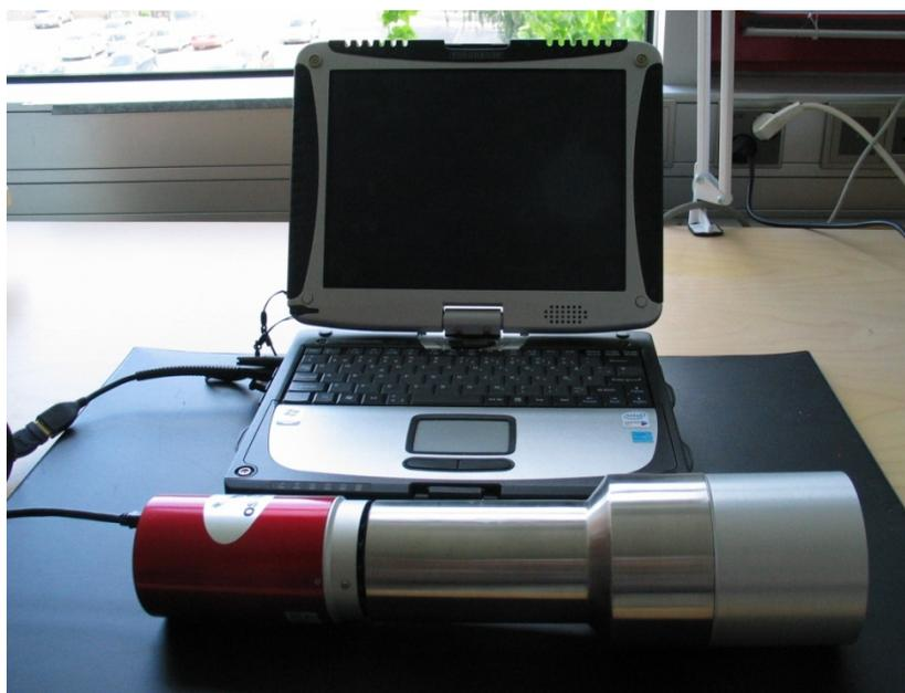
Figure 1. Capture-gated neutron spectrometer with laptop.
